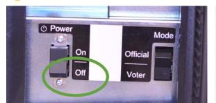
Using the barrel key, open the left side access compartment and flip the Power Switch to Off.
